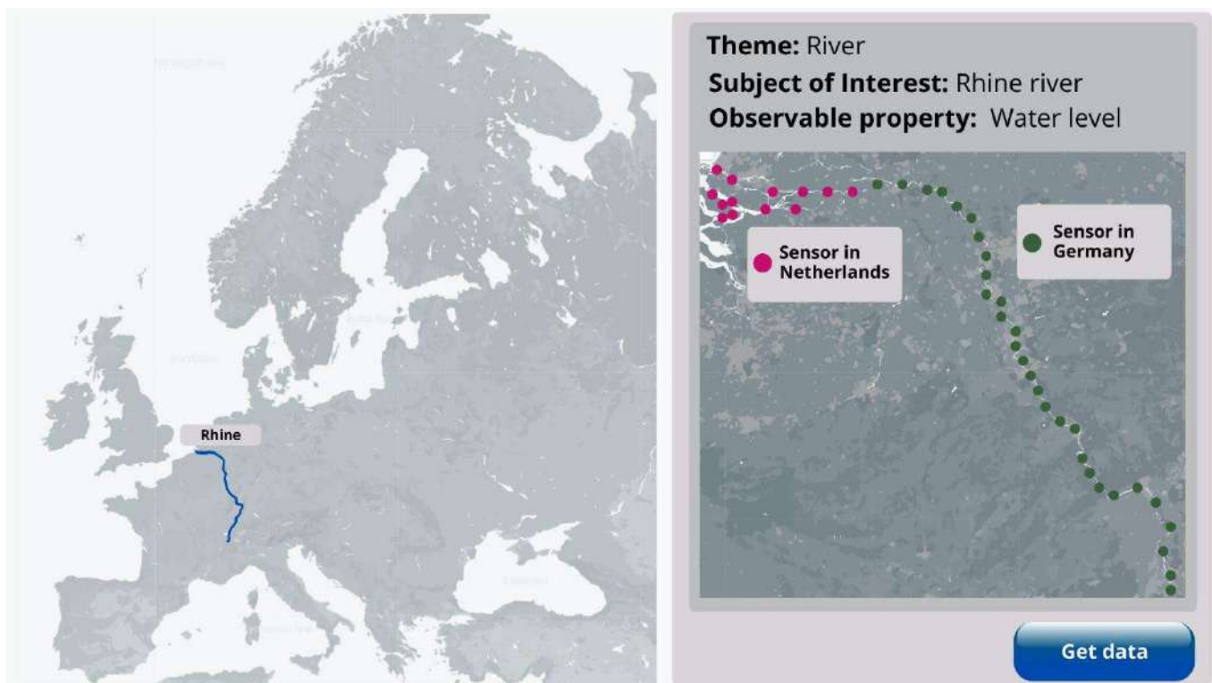
Figure 3 Selection of all station with the ability to observe waterlevel. The big difference between this scenario and the current situation is that it is now possible to retrieve data from already existing stations/sensors without caring about borders or ownership of the data.
